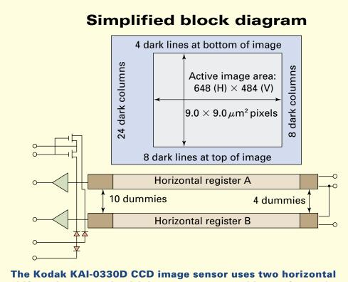
The Kodak KAI-0330D CCD image sensor uses two horizontal shift registers, each with its own output, to hit 120 frames/sec. A fast-dump feature permits quick dumping of unwanted rows to hit even higher frame rates for reading out a subsection of the full image. This feature lets the chip deliver two full-length rows at 400 frames/sec.
